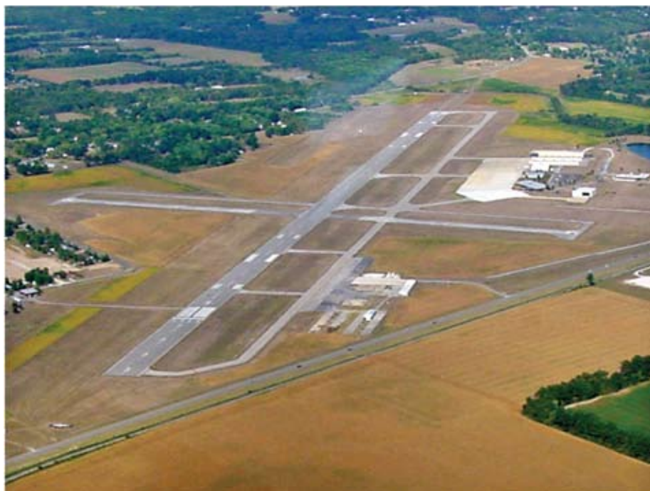
Mt. Vernon Outland Airport, Mt. Vernon, Illinois, was the "2007 Illinois Airport of the Year." The airport features a 6,500 ft. main runway, a crosswind runway, and an ILS approach.
