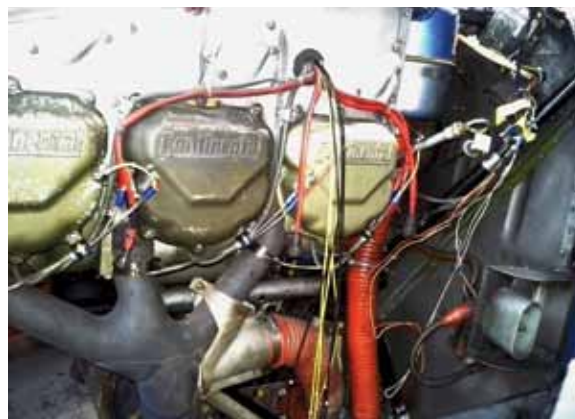
Installing the wiring to the cylinders. Gran-Aire Photo
