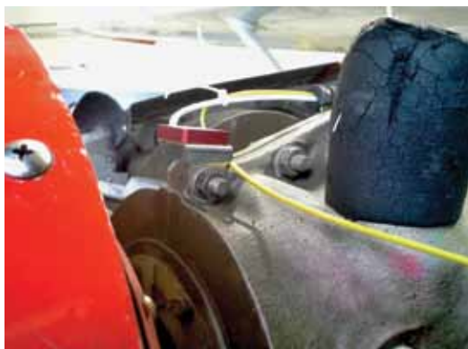
Engine vibration sensor. Gran-Aire Photo
