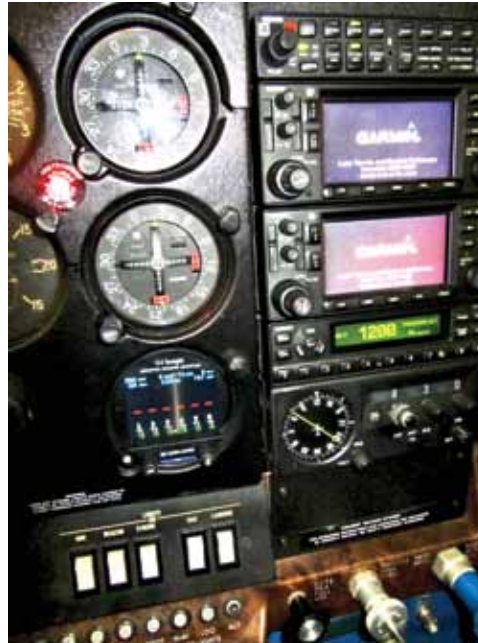
It is important to position the graphic engine monitor (lower left instrument) so information can be easily viewed while flying.
