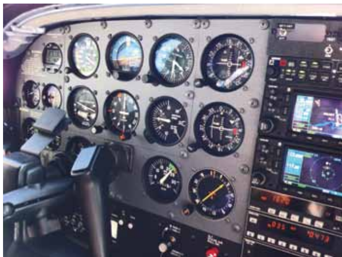
Fig 1: Two OBS indicators set to the same VOR with reciprocal settings.
